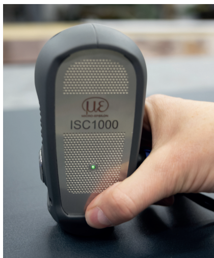
The ISC1000 uses microwave technology to measure the total layer thickness of insulating materials on CFRP and metal substrates in a non-destructive way without a coupling medium. © Micro-Epsilon
