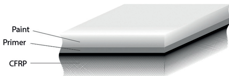
Typical structure of an aircraft paint coat. The coating thickness has an influence on weight, lightning protection, UV resistance and corrosion protection. © Micro-Epsilon
